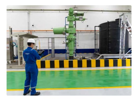
The all-electric surface actuator demonstrator enables remote valve operation and health monitoring savings costs by reducing visits to offshore platforms and remote locations.
